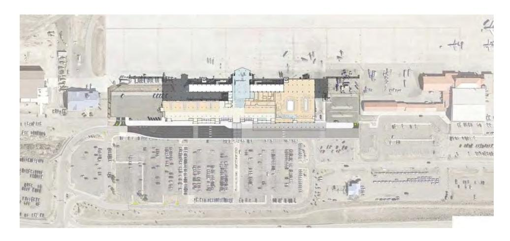
Expansion along the terminal loop roadway section adjacent to the terminal building creates four (4) traffic lanes; two (2) for stopping arrival and departure traffic and two (2) for vehicles passing that stopped traffic. Pedestrian crosswalks are reduced from five (5) to three (3) at critical locations. Access/egress for the commercial vehicle pickup lot is consolidated to a single location. Access/egress for the permit parking lot is also consolidated to a single location.
