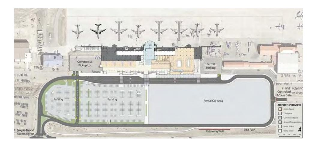
The existing terminal loop roadway is extended to the east allowing rental car facilities to be consolidated within the new loop road. This requires the creation of a retaining wall on the south side of the new road and a relocation of the existing bike path. An ACI gate is created on Eldon Wilson Road just east of the new terminal loop roadway.
