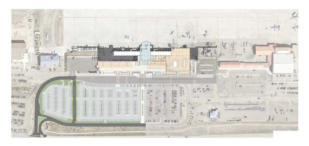
A commercial vehicle bypass lane is created through the existing short-term parking lot with direct access to the commercial vehicle pickup lot. Entry and exit locations for parking are reduced to one (1) each, both positioned to prevent parking vehicles from passing the terminal building along the loop road.
